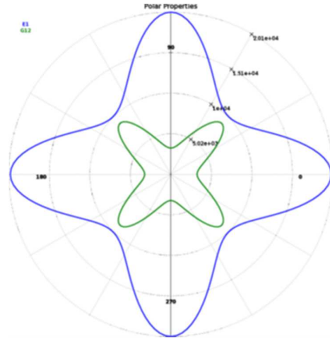
Figure 1. Young's and Kirchhoff's modules as a function of fibre direction for single layer of glass fabric.
