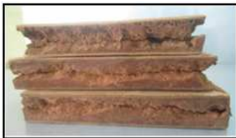
(c) Crushed sandwich with continuous cracks
