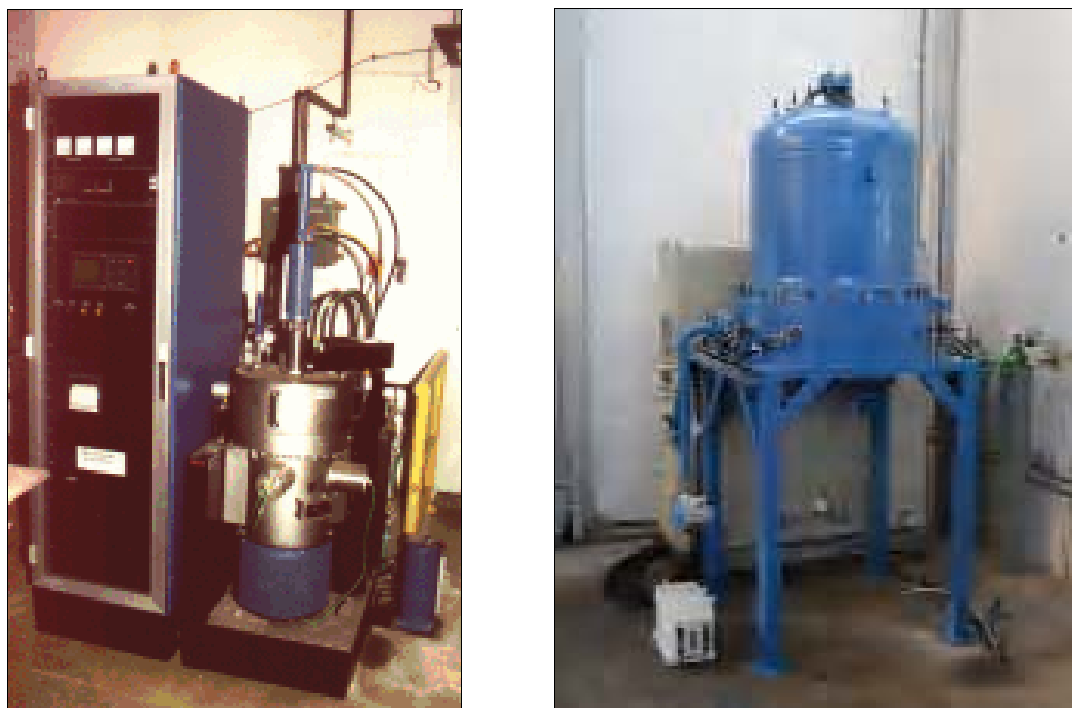
Fig. 2. High temperature autoclaves for the production of CF-Mg samples and for technology demonstrators
