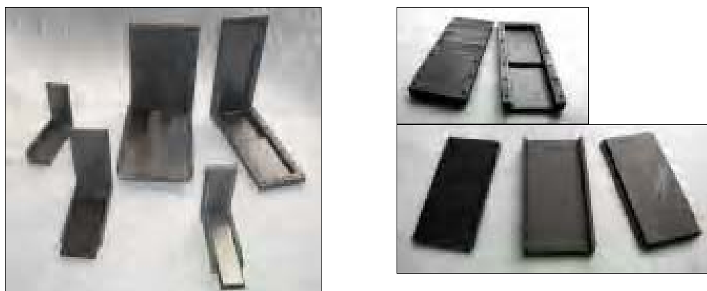
Fig. 3. Component graphite moulds for CF-Mg plates [4]
