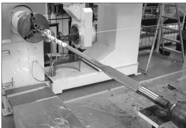
Fig. 12. Winding of transmission shaft on an 5-axis winding machine at ILK
