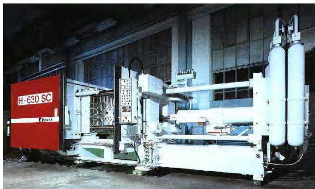
Fig. 7. BÜHLER real-time operating high pressure die casting machine
