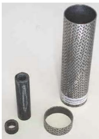
Fig. 10. Graphite form tools (a) and fabricated CF-Mg-tubes (b) [3]
