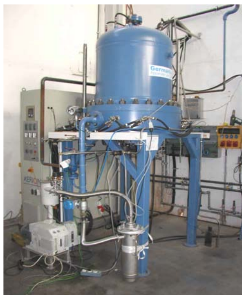
Fig. 9. High temperature autoclaves for the production of CF-Mg structures
