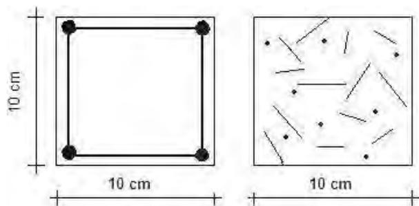
Fig. 1. Cross-section of concrete beams with aligned and short reinforcement distributed in volume unit
