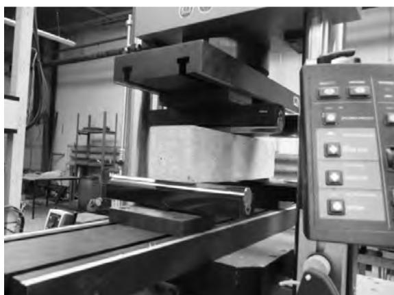
Fig. 4. Stand for testing beams
