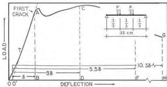
Fig. 3. Load-deflection curve according to standard [ASTM C1018]
