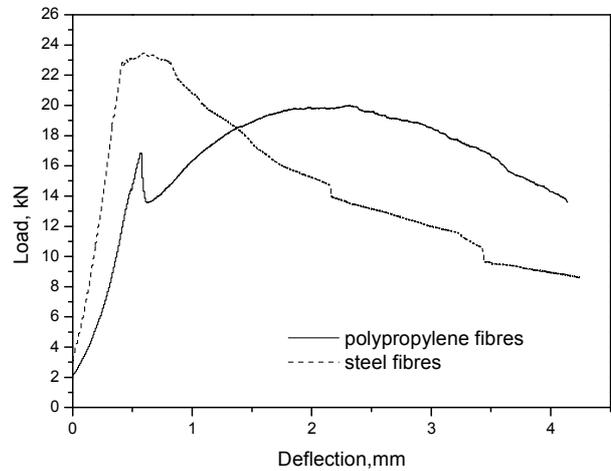
Fig. 11. Comparison of load-deflection curves for concrete beams reinforced with steel and polypropylene macro-fibres
