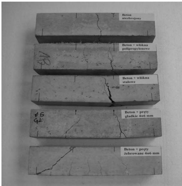
Fig. 10. Morphology of cracks in relation to different types of reinforcement
