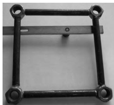
Fig. 2. Stirrup with slip sleeves in corners to enable proper interaction between steel rods and cement matrix
