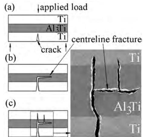
Fig. 4. Crack propagation in Ti-Al<sub>3</sub>Ti specimen loaded perpendicular to layers
