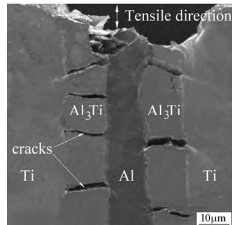
Fig. 2. Cross-section of fractured Ti-(Al<sub>3</sub>Ti+Al) tensile specimen showing metals layers bridging many cracks in aluminide layers
