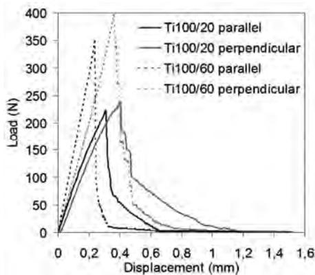
Fig. 3. Load-displacement curves of Ti100/20 and Ti100/60 specimens at different load directions during three-point bending test
