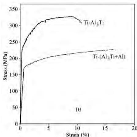
Fig. 1. Tensile curves for Ti-(Al<sub>3</sub>Ti+Al) and Ti-Al<sub>3</sub>Ti composites
