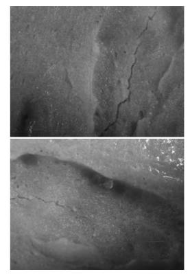
Fig. 1. Microcracks observed in PMMA directly after polymerization process
