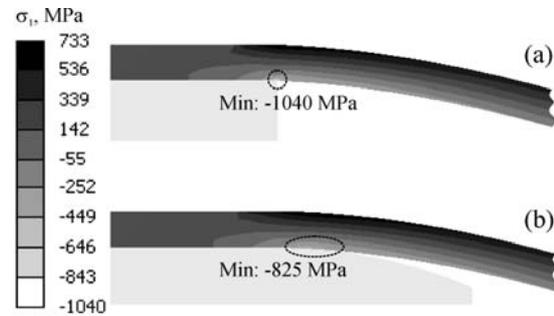
Fig. 7. Normal stress in fibre direction of unidirectionally reinforced GFRP-E specimens (thickness 9.5 mm) at a deflection of 60 mm with supporting radius of (a) 0 mm and (b) 125 mm
