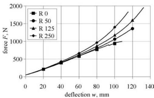
Fig. 6. Force-deflection diagram of GFRP-E specimens with thickness of 9.5 mm for different supporting radii
