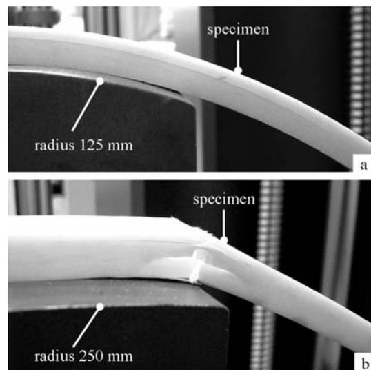
Fig. 8. Deformation of GFRP-E specimens (thickness 9.5 mm) for supporting radius of (a) 125 mm and (b) 250 mm
