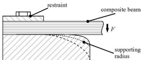
Fig. 3. Load transfer element with adaptable supporting radius
