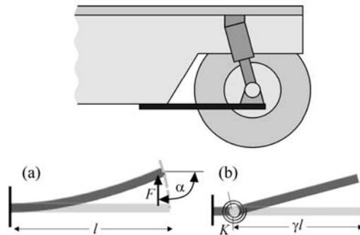
Fig. 1. Chassis component and associated simplified mechanical model of a cantilever beam; (a) applied force  $F$  and associated angle  $\alpha$  and (b) PRBM with characteristic radius factor  $\gamma(\alpha)$  and characteristic spring constant  $K(\alpha)$  [15]
