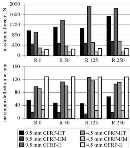
Fig. 5. Maximum force and associated deflection of specimens with different composite materials and thicknesses (maximum deflection of test rig reached for GFRP-E, thickness 4.5 mm)
