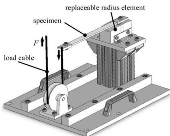
Fig. 4. CAD-model of test rig with pull cable mechanism ensuring vertical load
