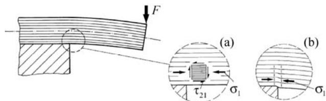
Fig. 2. Superimposed shear and compressive stresses at end of load transfer element; (a) local loading condition and (b) deformation due to shear stress promotes fibre kinking [16]
