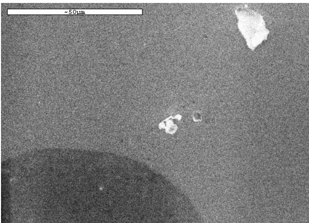
Fig. 6. SEM image of Ni-graphene coating. Sample 4. Graphene particle in nickel coating
