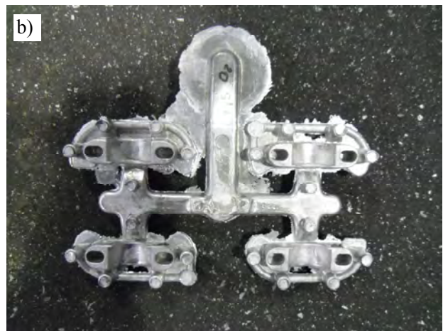
Fig. 2. Composite casts after removal from pressure die cast machine: a) samples for mechanical properties examination, b) composite products
