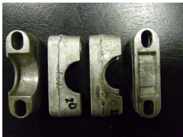
Fig. 3. Macrograph of Mg3Al-GCp composite casts after trimming procedure
