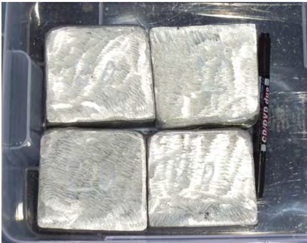
Fig. 1. Composite ingots cleaned by abrasive machining applied for preparation of secondary suspension
