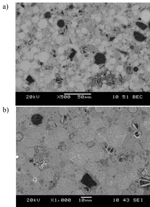
Fig. 2. SEM image of  $\text{TiB}_2\text{-TiN}$  composite obtained with HP-HT method from nanopowders: a) magnification of 500x BEC, b) magnification of 1000x, SEI
