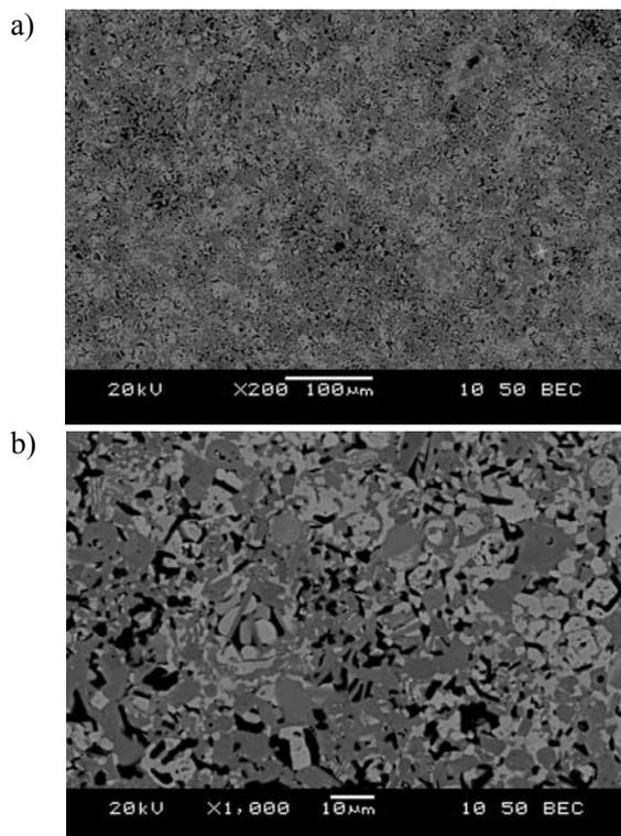
Fig. 3. SEM image of TiB<sub>2</sub>-TiN composite obtained using SPS method from nanopowders: a) magnification of 200x, BEC, b) magnification of 1000x, BEC
