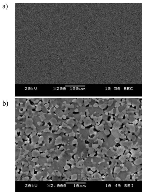
Fig. 4. SEM image of TiB<sub>2</sub>-TiN composite obtained using SPS method from micropowders: a) magnification of 200x, BEC, b) magnification of 2000x, SEI
