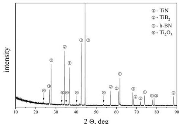
Fig. 5. X-ray diffraction diagram of TiB<sub>2</sub>-TiN(2) composite obtained using SPS method from nanopowders
