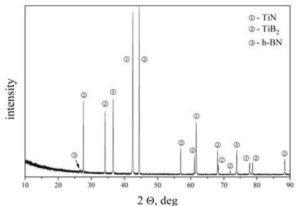
Fig. 6. X-ray diffraction diagram of TiB<sub>2</sub>-TiN(3) composite obtained using SPS method from micropowders
