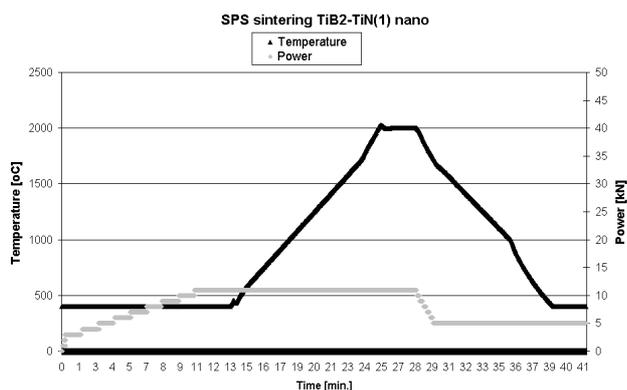
Fig. 1. Example of SPS sintering curve for sample  $\text{TiB}_2\text{-TiN}(1)$ , in Table 3
