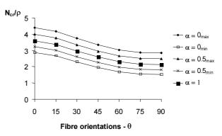
Fig. 6. Distributions of buckling loads for compressed angle-ply plates
