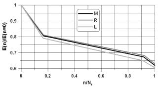
Fig. 4. Degradation of laminate (glass fiber/epoxy resin) stiffness vs. number of cycles (mean values - M, upper - R and lower - L bounds, respectively)
