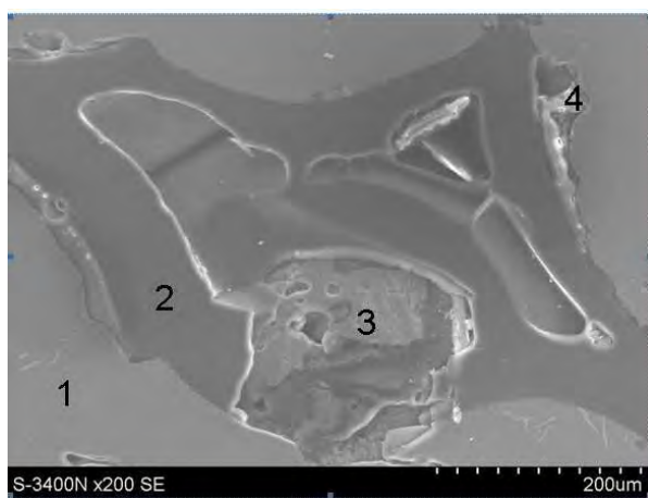
Fig. 10. Phase boundary in composite containing carbon foam with porosity of 85%: 1 - matrix, 2 - carbon foam wall, 3 - carbon cell not filled up with matrix material, 4 - discontinuity on phase boundary
