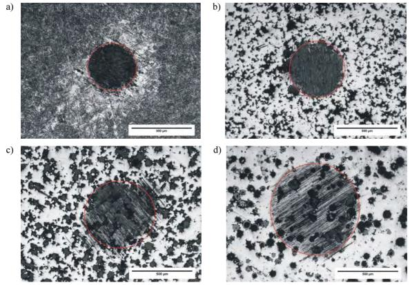
Fig. 5. Microscope photographs of wear on specimen surface: a) 100% Ti-6Al-4V, b) 80% Ti-6Al-4V + 20% Al<sub>2</sub>O<sub>3</sub>, c) 80% Ti-6Al-4V + 20% HAp, d) 80% Ti-6Al-4V + 20% YSZ
