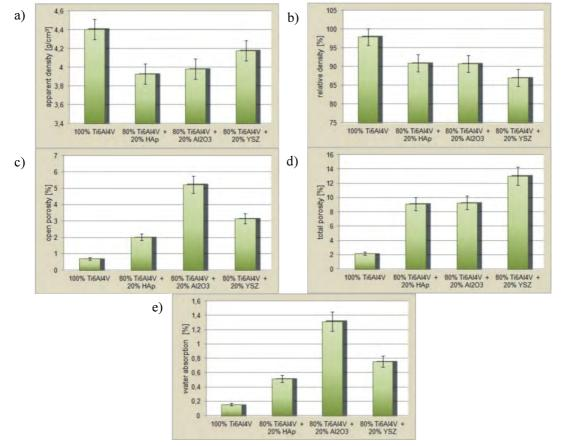
Fig. 3. Graph of: a) apparent density, b) relative density, c) open porosity, d) total porosity, e) water absorption of metallic-ceramic sinters
