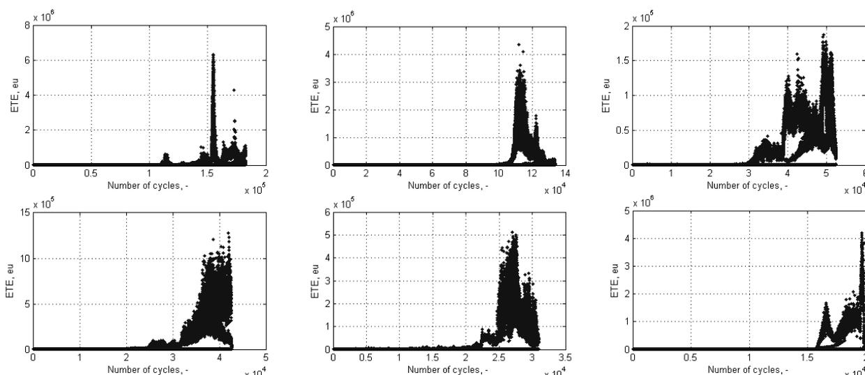
Fig. 4. AE energy ratios for selected fatigue tests for considered values of stabilization temperature
