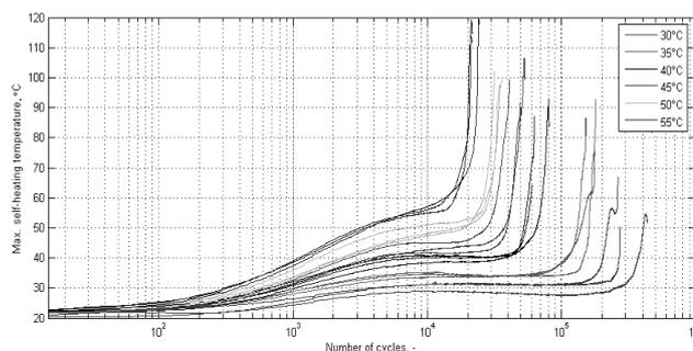
Fig. 2. Selected self-heating temperature history curves for various stabilization temperature values
