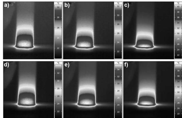
Fig. 3. Thermograms of tested specimens after various numbers of cycles: with self-heating stabilization temperature of 30°C after: a) 103455, b) 275355, c) 386835 cycles and stabilization temperature 35°C after d) 16380, e) 147570, f) 187095 cycles
