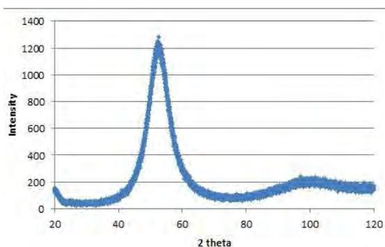
Fig. 4. Diffraction pattern of Ni-P layer
