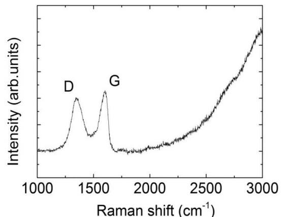
Fig. 2. Raman spectrum of graphene flakes
