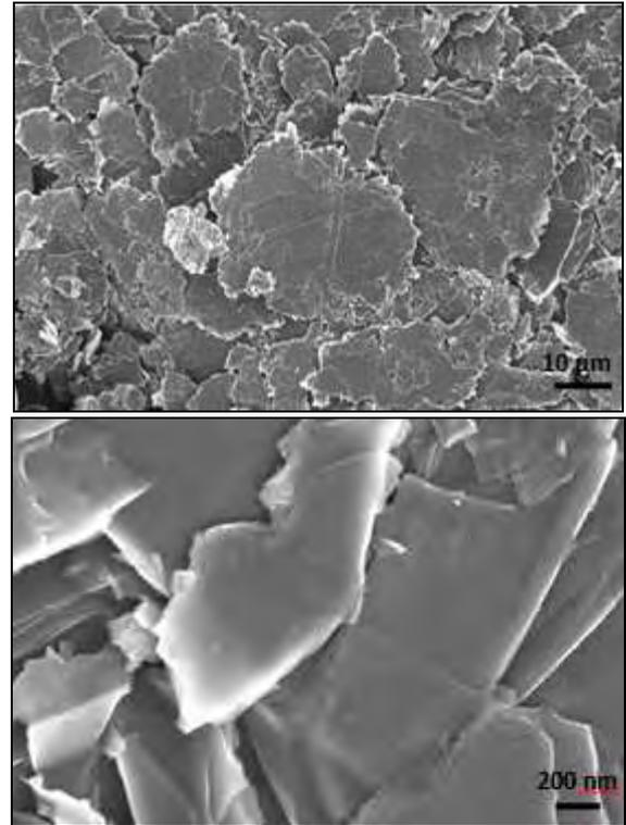
Fig. 1. Images (SEM) of graphene flakes
