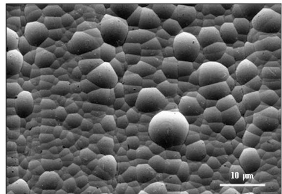
Fig. 3. Image (SEM) of morphology and topography of Ni-P layer
