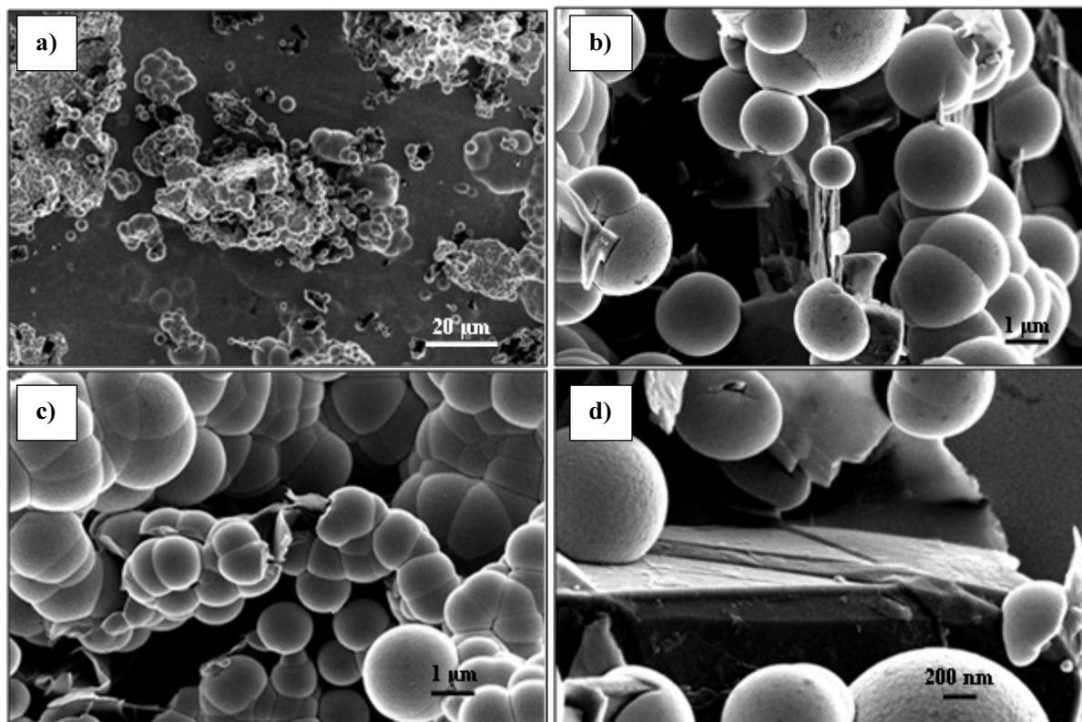
Fig. 5. Images (SEM) of Ni-P/G layer surfaces: a) surface topography, b-d) graphene flakes incorporated into Ni-P matrix
