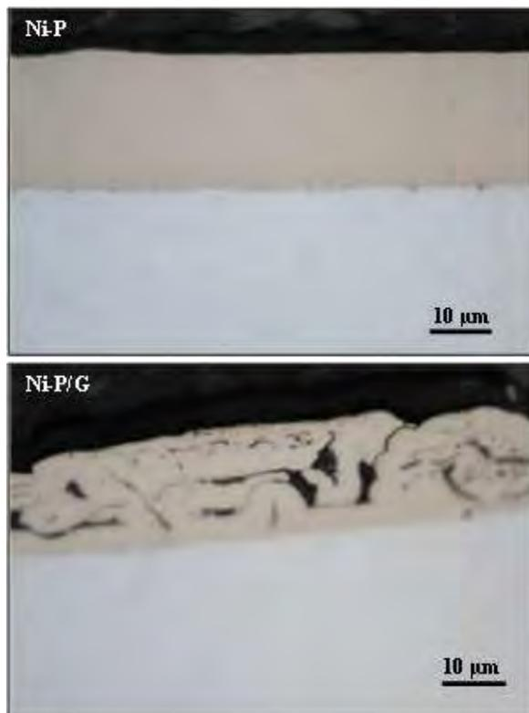
Fig. 7. Cross sections of surface layers of Ni-P and Ni-P/G with graphene aggregates in Ni-P matrix
