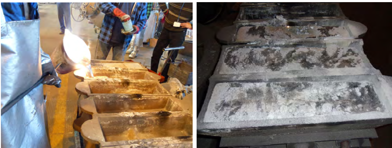
Fig. 5. Pouring suspension from hand shank into open steel moulds (a), suspension during crystallization in steel moulds (b)
