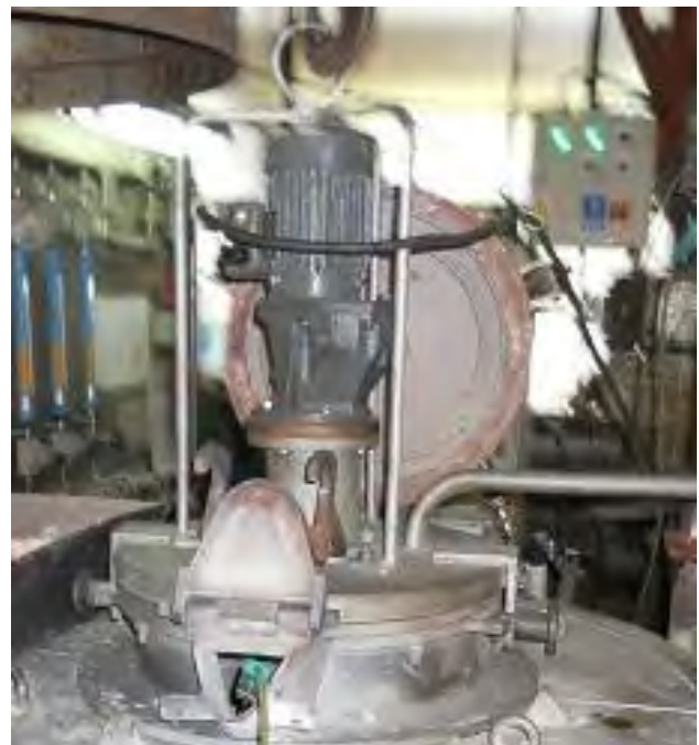
Fig. 3. Electric furnace with mixing system applied for suspension fabrication
