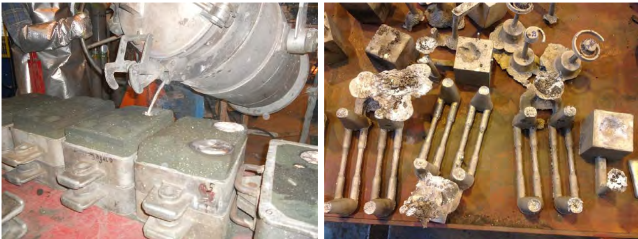
Fig. 4. Pouring suspension from thermos into ceramic moulds (a), obtained composite casts after fettling (b)
