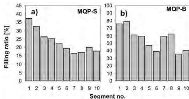
Fig. 7. Variation of filling ratio along gear radius in gear produced with (a) spherical powder, and (b) 'flaky' powder
