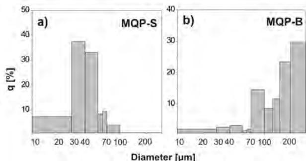
Fig. 3. Particle size distributions in MQP-S powder (a) and MQP-B powder (b)
