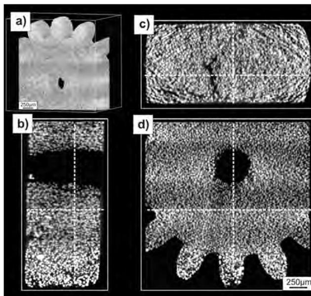
Fig. 4. Images (X-ray tomography) of miniature magnetic gear produced from MQP-S powder (a) and images of its cross-sections analyzed in the study (b, c, d)
