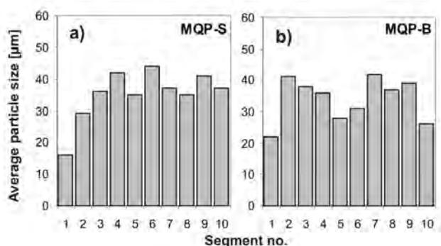
Fig. 8. Variation of average particle size along radius of gear produced with 'spherical' powder (a) and 'flaky' powder (b)
