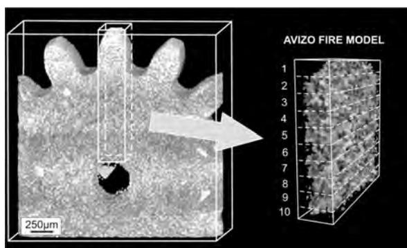
Fig. 6. Image of cross-section of gear showing places where it was cut out (numbers refer to sectors selected for calculating filling ratio and average particle size)
