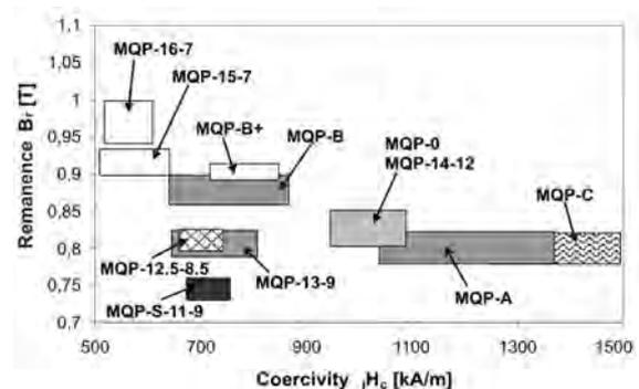
Fig. 2. Remanence and coercivity of high-coercivity powders produced by Magnetquench Co. Symbols given in the figure are trade marks of the powders (from: [www.magnetquench.com](http://www.magnetquench.com))
