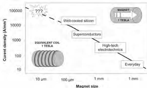
Fig. 1. Electric current density necessary to generate magnetic field of 1 T depending on coil dimensions, compared to that of permanent magnet of same size
