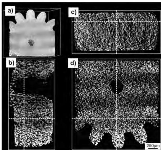
Fig. 5. Images (X-ray tomography) of miniature magnetic gear produced from MQP-B powder (a) and images of cross-sections of this gear (b, c, d)
