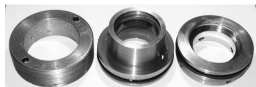
Fig. 3. Packing nut (left), stuffing-box with guide rings made of PTFE composite in closed groove (central), stuffing-box with opened groove of seal and leakage holes (right) [2]
