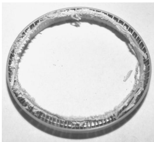
Fig. 4. Mupuseal 30412 - 0450 - 90 - S seal after 20 000 m of friction distance. Visible wear products on the seal from the guide elements made of UHMWPE [1]
