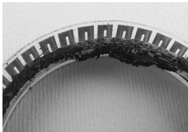
Fig. 5. Mupuseal 30413 - 0450 - 90 - S seal after 90 000 m of friction distance. Visible wear products on the seal from the guide elements made of Kefloy-22
