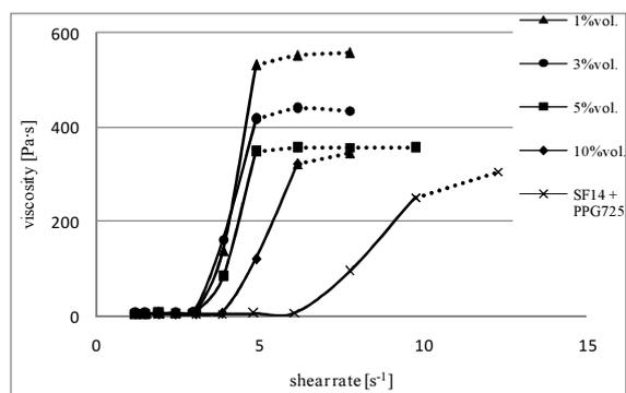
Fig. 7. Viscosity curves of STF based on SF14 doped by modified halloysite dispersed in PPG 725
