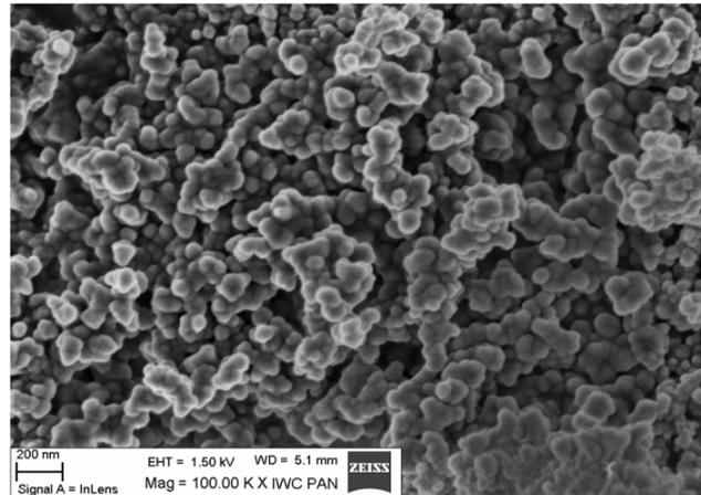
Fig. 1. Nanosilica microstructure
