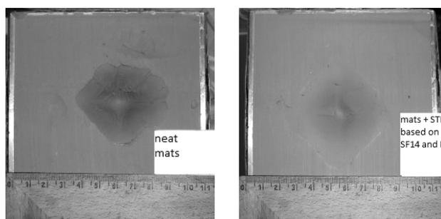
Fig. 8. Photographs of deformations in ballistic plasticine
