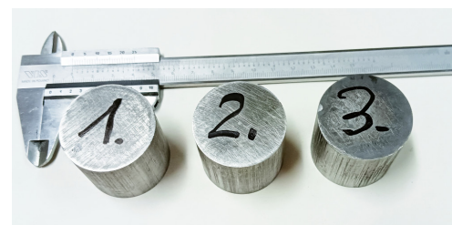
Fig. 2. Hot-compact samples of AA2024/SiC composite
