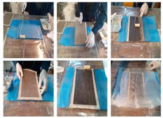
Fig. 2. Sequence of lamination phases
