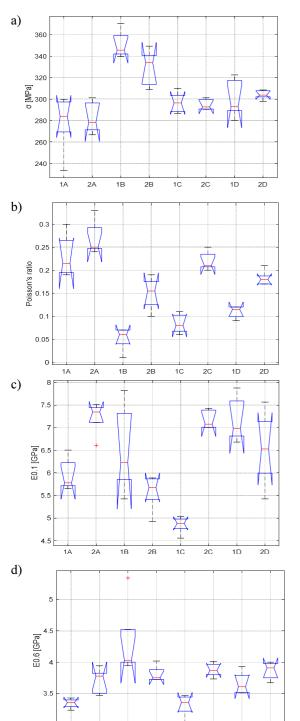
Fig. 9. Box plots of mechanical properties for all tested species: a) tensile strength  $\sigma$ ; b) Poisson's ratio; c) elastic modulus for 0.1 N/N<sub>max</sub>; d) elastic modulus for 0.6 N/N<sub>max</sub>
