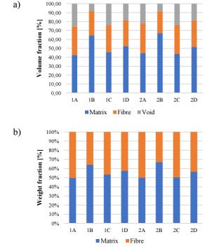
Fig. 4. Histograms of: a) volume percentage of matrix, fibres and voids, b) weight percentage matrix and fibre of all produced composites
