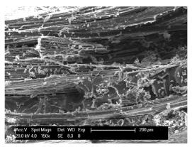
Fig. 8. SEM micrograph of fracture surface of 1B2 specimen after tension test
