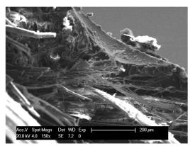
Fig. 7. SEM micrograph of fracture surface of 1A2 specimen after tension test
