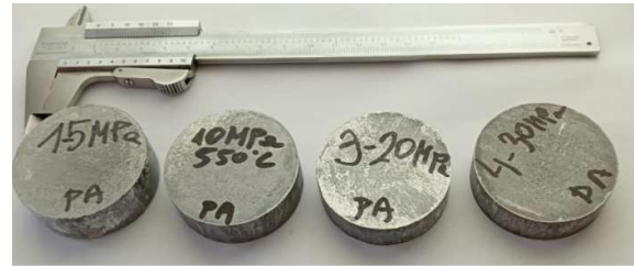
Fig. 3. Hot-pressed AA2024/fly ash specimens at 550 °C and 5, 10, 20, 30 MPa pressure
