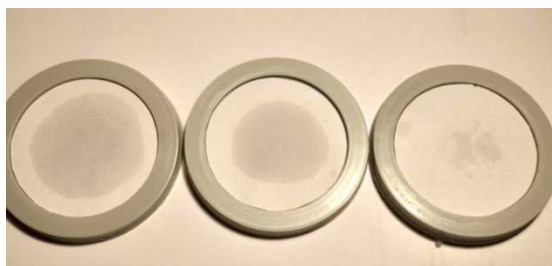
Fig. 2. Leakage of composite paraffin, from left: vacuum impregnated 1:5, immersion impregnated, vacuum impregnated 1:3
