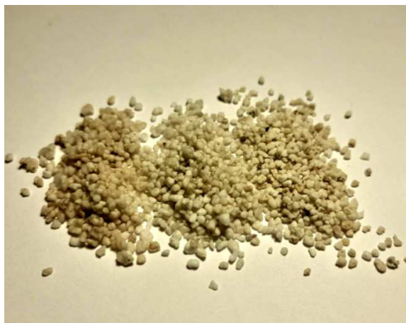
Fig. 1. Perlite:paraffin composites, from left: vacuum impregnated 1:5, immersion impregnated, vacuum impregnated 1:3
