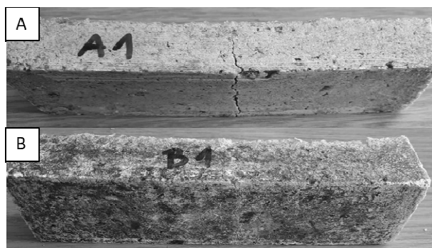
Fig. 7. Samples after three-point bending test. A – A sample, B – series B sample
