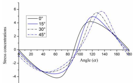
Fig. 5. Stress concentrations  $\sigma_\alpha/S$  versus  $\alpha$  for four layered glass/epoxy composite
