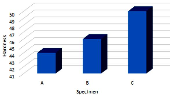
Fig. 5. Comparison of hardness of specimens: a) AZ91D, b) AZ91D+3% B<sub>4</sub>C, c) AZ91D + 2% ZrO<sub>2</sub> + 3% B<sub>4</sub>C
