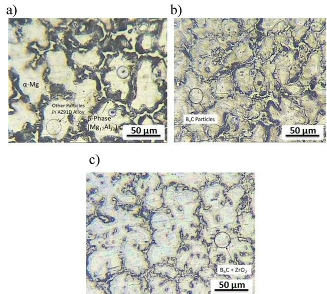
Fig. 4. Microstructure of: a) AZ91D, b) AZ91D+3% B<sub>4</sub>C, c) AZ91D+2% ZrO<sub>2</sub> + 3% B<sub>4</sub>C (recorded at 200 × magnification)
