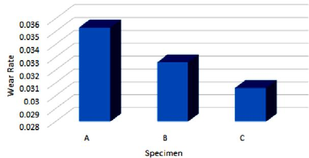
Fig. 6. Wear rate comparison of specimens: a) AZ91D, b) AZ91D+3% B<sub>4</sub>C, c) AZ91D+3% B<sub>4</sub>C+2% ZrO<sub>2</sub>
