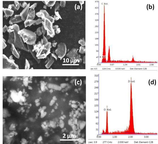
Fig. 3. SEM and EDS analysis of reinforcements: a) SEM micrograph of B<sub>4</sub>C, b) EDS analysis of B<sub>4</sub>C, c) SEM micrograph of ZrO<sub>2</sub> and d) EDS of ZrO<sub>2</sub>
