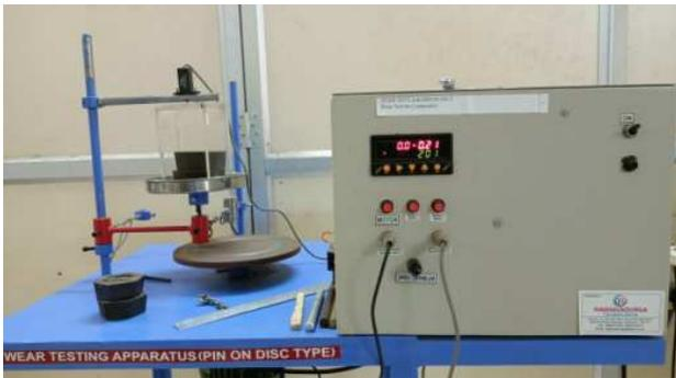
Fig. 2. Pin-on-disc equipment
