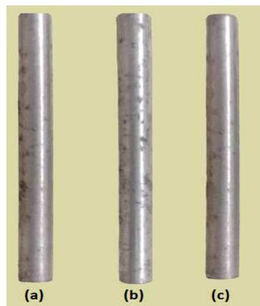
Fig. 1. Produced composite samples: a) AZ91D, b) AZ91D+3%B<sub>4</sub>C, c) AZ91D+3%B<sub>4</sub>C+2%ZrO<sub>2</sub>
