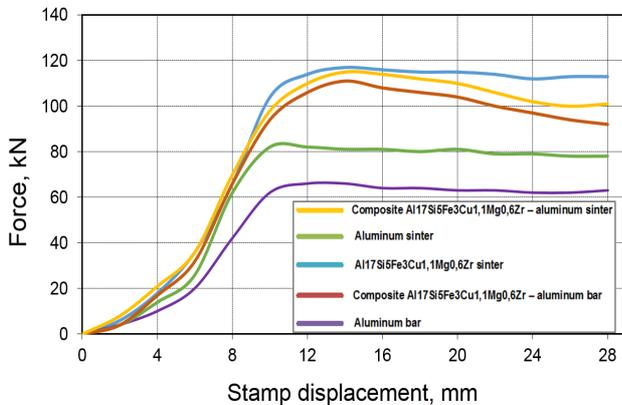
Fig. 4. Extrusion curves of component materials and bimetallic composites
