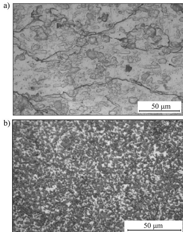
Fig. 5. Microstructures of component materials obtained by hot sintering under pressure of powders: a) aluminum and b) Al17Si5Fe3Cu1.1Mg0.6Zr alloy
