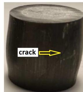
Fig. 8. Failed bimetallic composite sample in non-standard compression test
