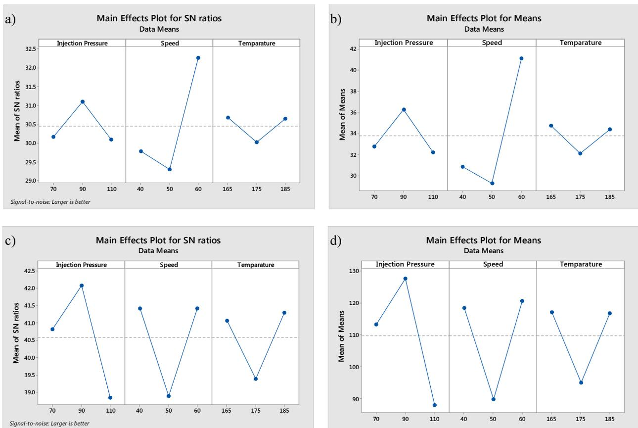
Fig. 4. Main effect plots of JF/PLA composite tensile strength (a-b) and flexural strength (c-d)
