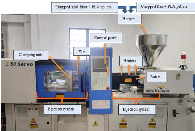
Fig. 3. Injection moulding machine used to fabricate the test specimens
