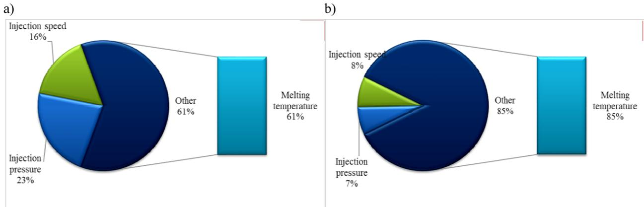
Fig. 7. Contribution of injection parameters on tensile (a) and flexural strength (b) of SF/PLA composite
