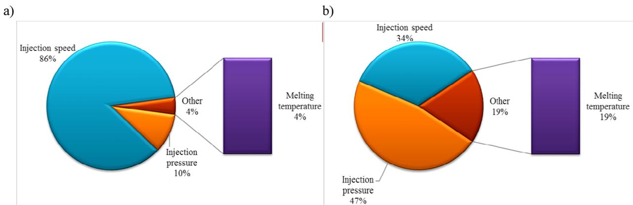
Fig. 5. Contribution of injection parameters on tensile (a) and flexural strength (b) of JF/PLA composite
