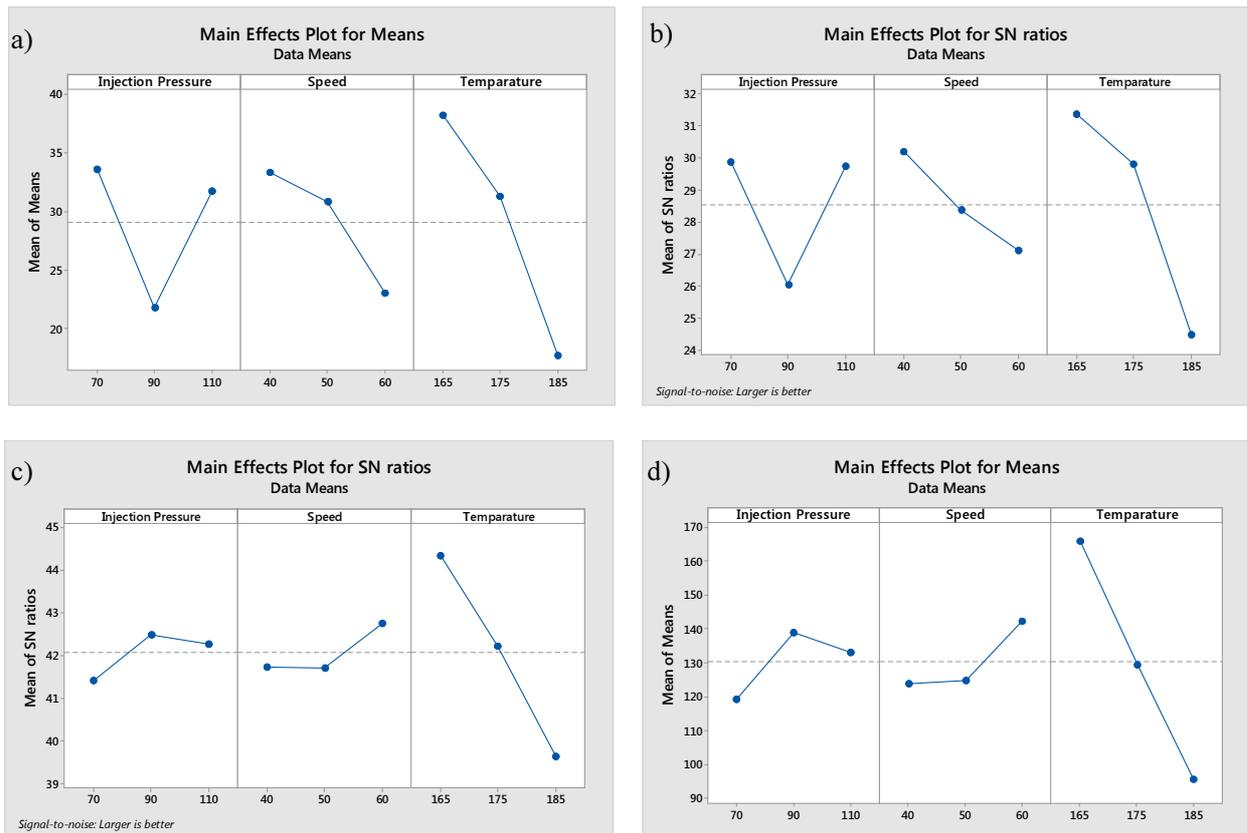
Fig. 6. Main effect plots of SF/PLA composite tensile strength (a-b) and flexural strength (c-d)
