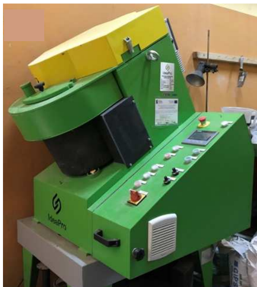
Fig. 1. Counter-current high intensity mixer used for the studies (Ideapro, Nowa Sól, PL)
