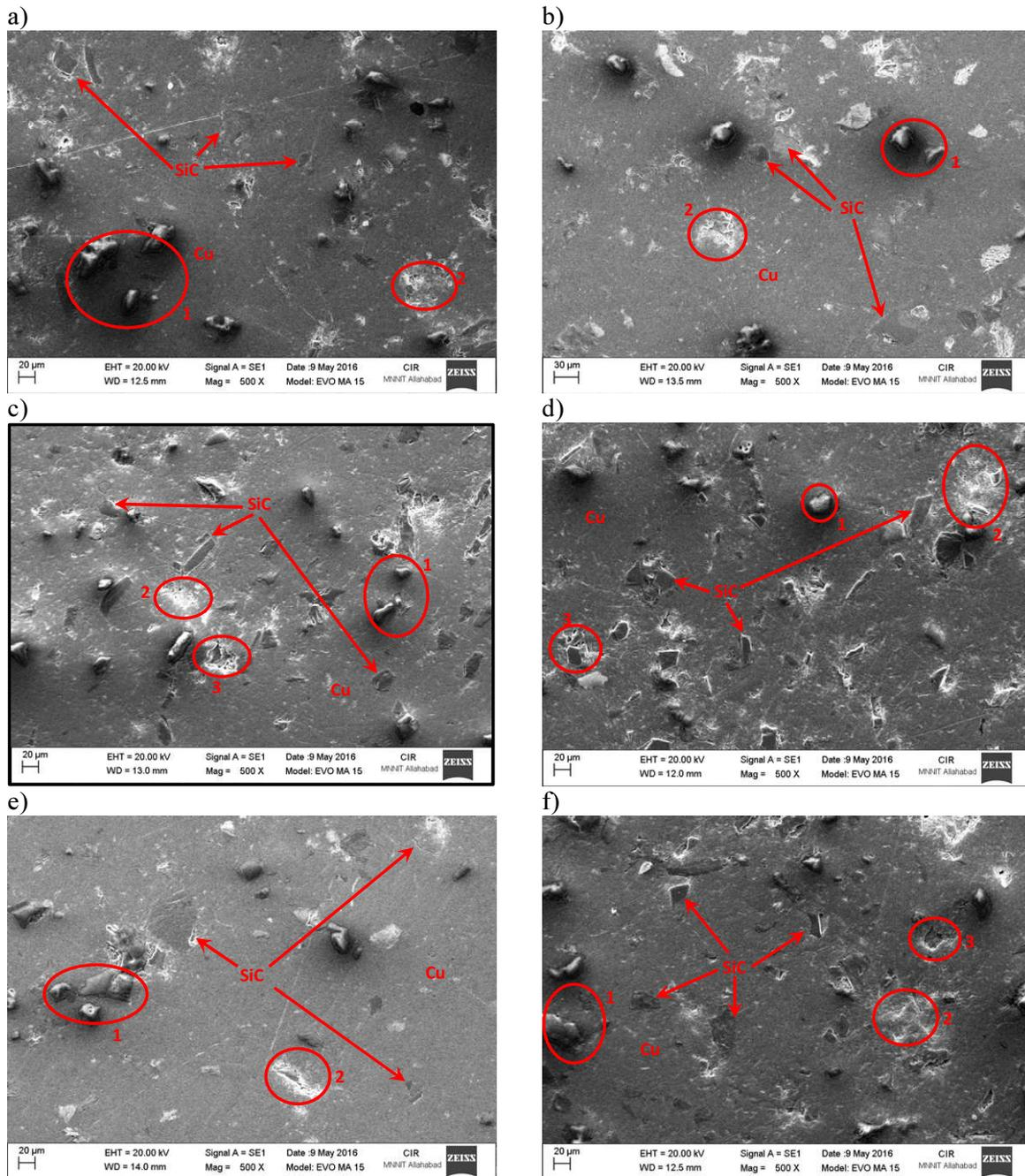
Fig. 2. SEM micrographs of (a) Cu-94.9 wt.%, SiC-5 wt.% and Cu wireframe structure 0.1 wt.% (b) Cu-94.8 wt.%, SiC-5 wt.% and Cu wireframe structure 0.2 wt.% (c) Cu-92.9 wt.%, SiC-7 wt.% and Cu wireframe structure 0.1 wt.% (d) Cu-92.8 wt.%, SiC-7 wt.% and Cu wireframe structure 0.2 wt.% (e) Cu-95 wt.% and SiC-5 wt.%. (f) Cu-93 wt.% and SiC-7 wt.%
