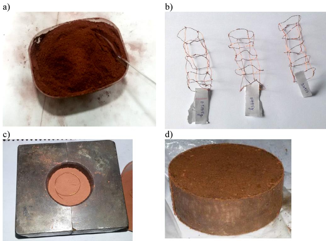
Fig. 1. Copper powder and SiC particle mixture with binder (a), copper wireframe structure (b), prepared mixture with wireframe structure in die before cold compaction (c), sample after sintering (d)
