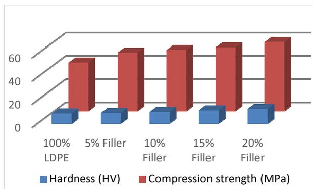
Fig. 3. Results of hardness and compressive strength of composite specimens
