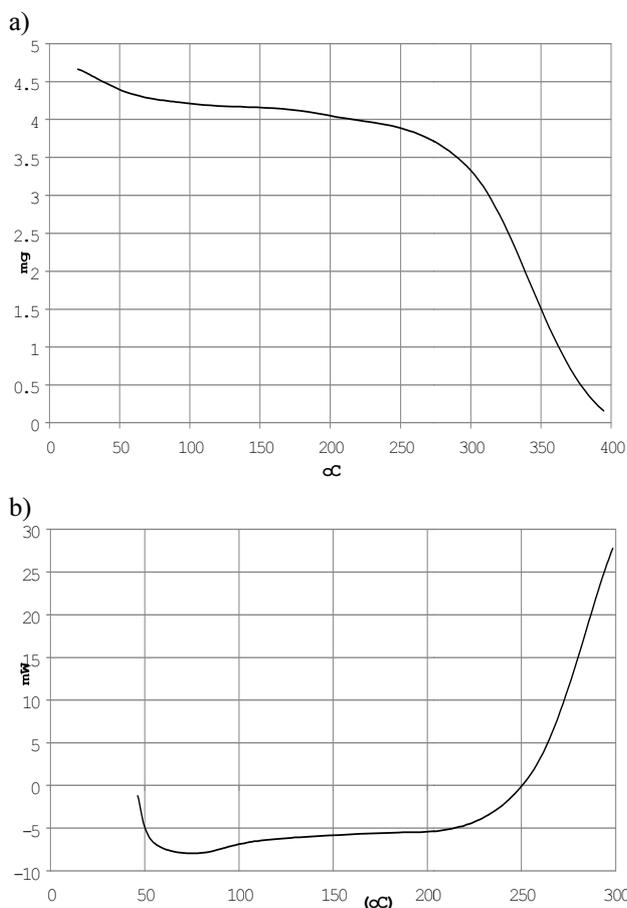
Fig. 2. Results of thermal analyses of filler: a) thermogravimetric analysis, and b) differential scanning calorimetry
