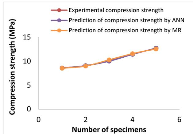
Fig. 5. Error comparison between MR and ANN for predicting compression strength of produced composites
