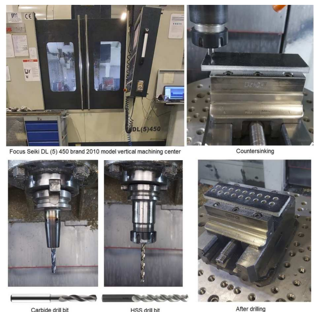
Fig. 2. Images of drilling process of GFRP composite material
