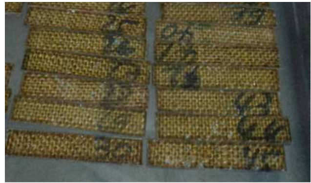
Fig. 1. Jute/polyester (JP) composite test pieces immersed in water
