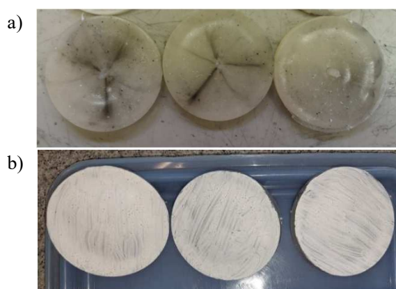
Fig. 2. Samples with BaSO 4 : neat (a) and coated (b)
