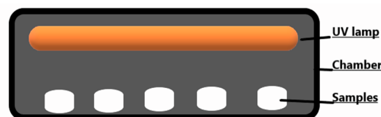
Fig. 3. Diagram of sample exposure in UV-chamber
