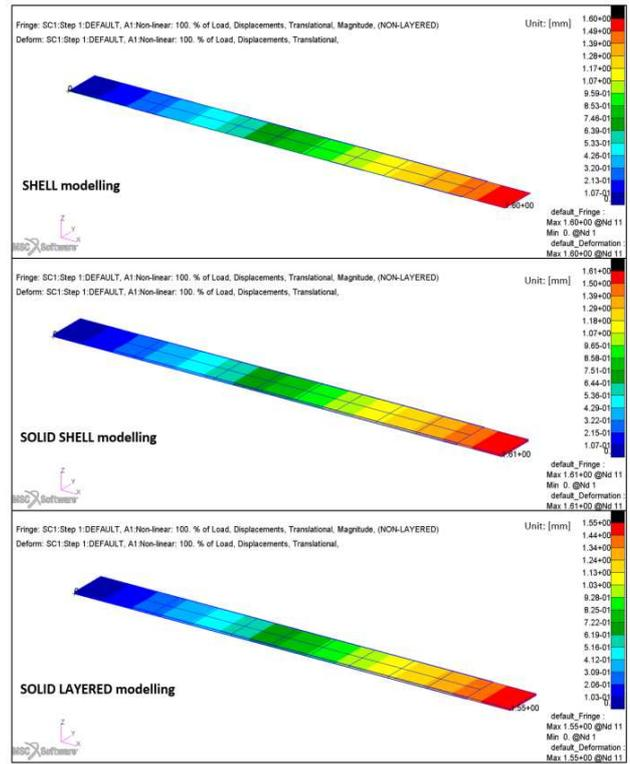
Fig. 18. Displacements for Model no. 1 in tensile FEAs: shell, solid shell, solid layered FE modelling
