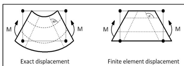
Fig. 6. Isoparametric lines for bending – diagram (authors' own elaboration)
