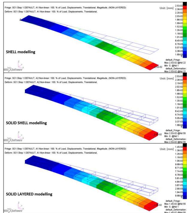
Fig. 14. Displacements for Model no. 3 in bending FEAs: shell, solid shell, solid layered FE modelling
