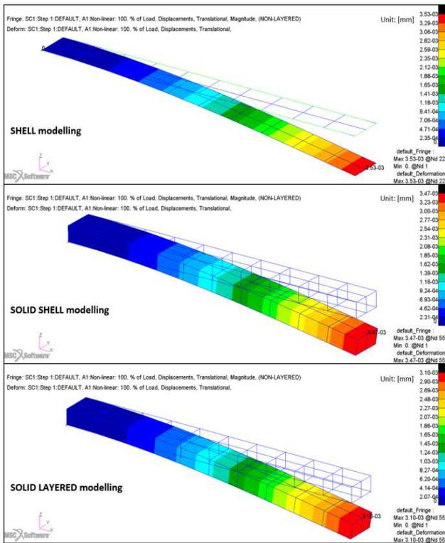
Fig. 16. Displacements for Model no. 4 (sandwich structure) in bending FEAs: shell, solid shell, solid layered FE modelling
