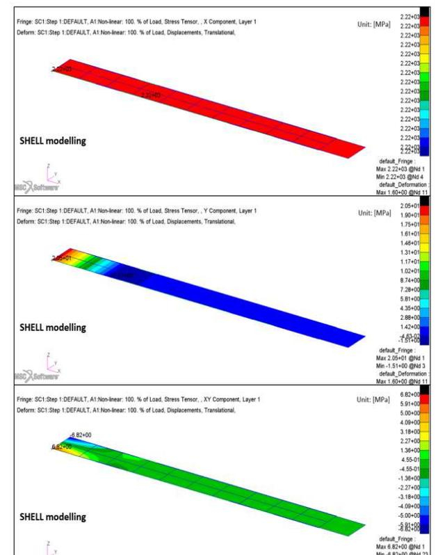
Fig. 19. X, Y stress components and XY stress for Model no. 1 in tensile FEAs: shell modelling
