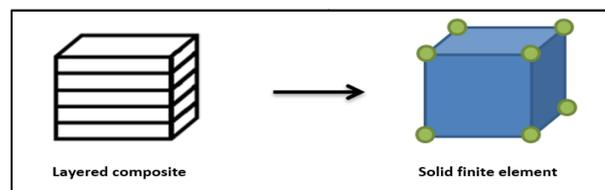
Fig. 3. Solid layered composite modelling
