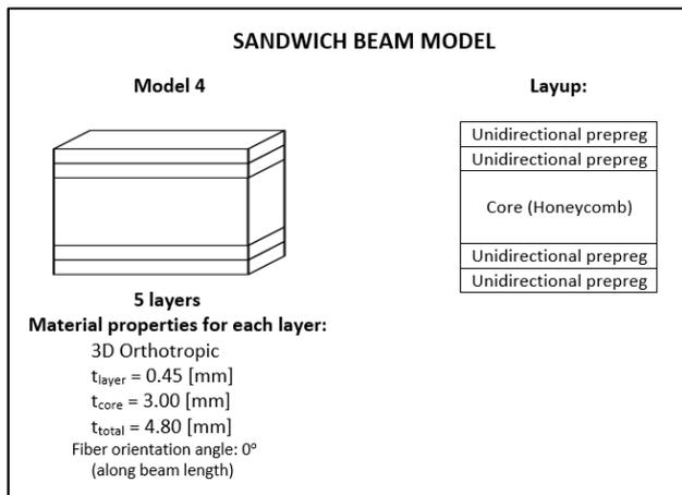
Fig. 13. Parameters of sandwich beam model
