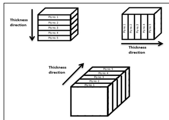
Fig. 4. Definition of orientation of plies in solid layered composite modelling
