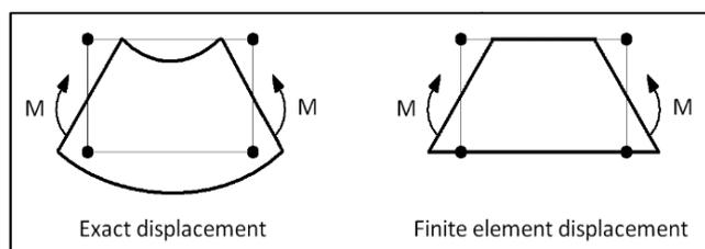
Fig. 5. Exact and finite element displacement in bending – diagram (authors' own elaboration)
