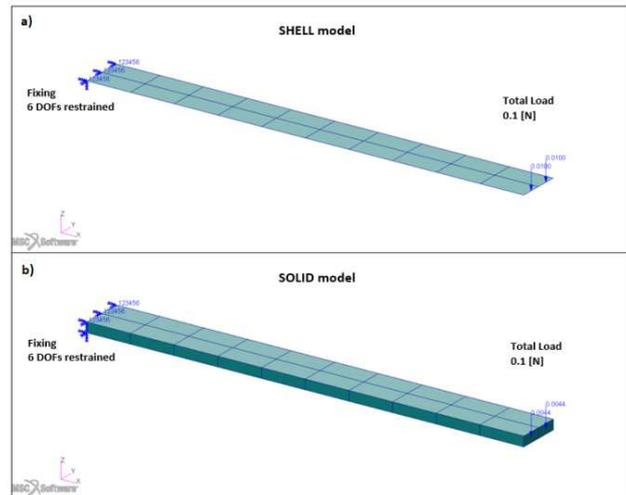
Fig. 10. Beam shell (a) and solid (b) FE model in bending
