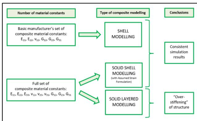
Fig. 20. Choice of composite finite element modelling type based on number of composite material constants
