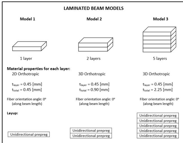
Fig. 12. Parameters of laminated beam models
