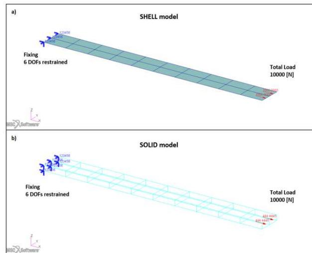
Fig. 11. Beam shell (a) and solid (wireframe view) (b) FE model in tension
