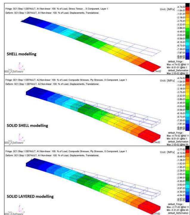
Fig. 15. X stress component for Model no. 3 in bending FEAs: shell, solid shell, solid layered FE modelling
