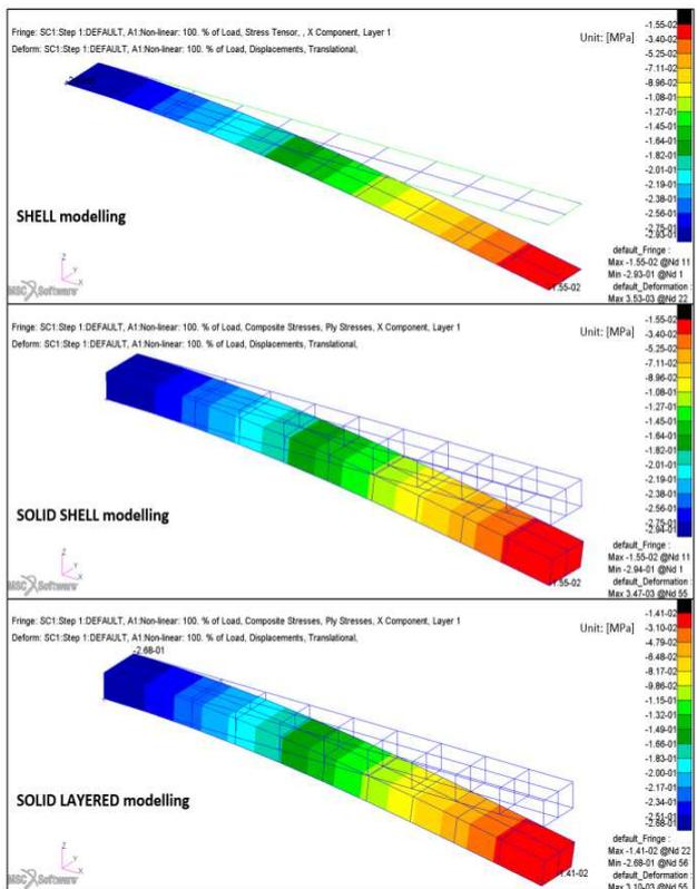
Fig. 17. X stress component for Model no. 4 (sandwich structure) in bending FEAs: shell, solid shell, solid layered FE modelling
