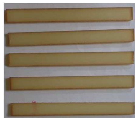
Fig. 2. TiO 2 NTs/epoxy composite flexural test specimens
