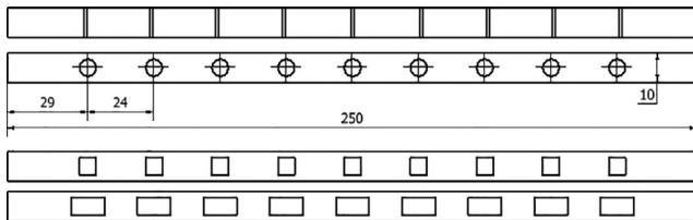
Fig. 1. Diagrams of milled defects with characteristic dimensions of tested specimens [7]
