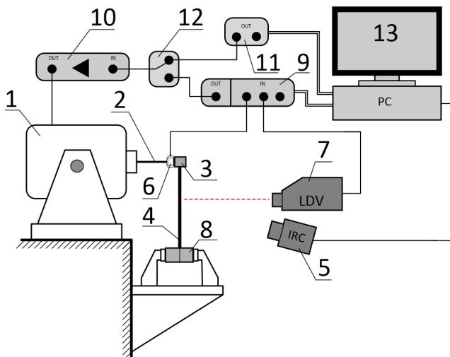
Fig. 2. Diagram of experiment test rig [7]
