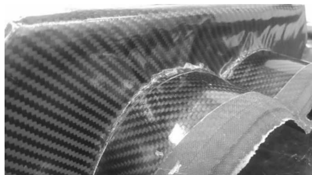
Fig. 12. Inaccuracy of adhesion of outer layers in bend area with small radius of curvature
