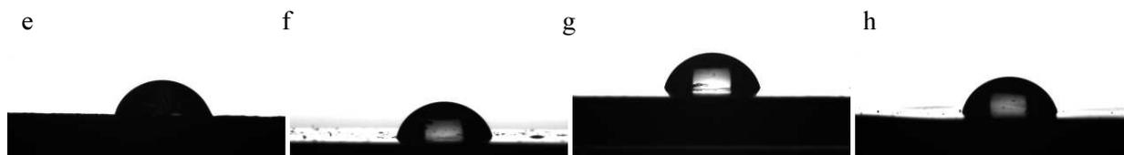
Fig. 9. Photographs of water droplets on polyurea compositions after 5 days of conditioning at 80°C (e-h), from left: e) reference, f) Sample A, g) Sample B, h) Sample C
