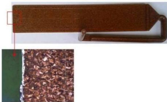
Fig. 1. Molded piece sample made of wood-polymer composite with enlarged area showing variable shape of wood fibers
