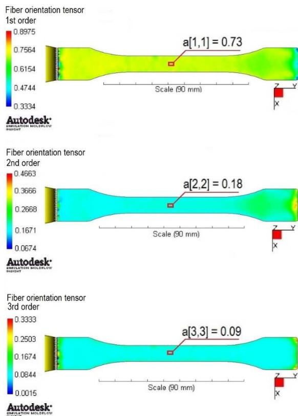
Fig. 5. Calculated fiber orientation tensor values (1-, 2-, 3-order) in chosen areas of specimen (10% WF)
