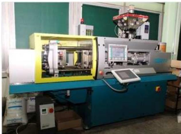
Fig. 2. Dr Boy 55E injection molding machine used in the research
