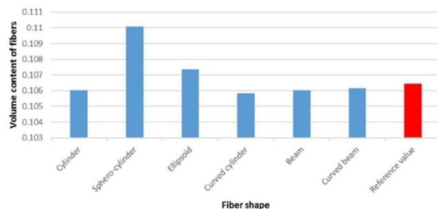
Fig. 6. Calculated volume content of fibers in analyzed RVE (for reference fiber content of 0.106445 set as input value)
