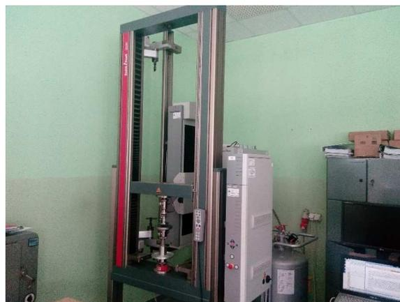
Fig. 4. Zwick Roell Z030 materials testing machine used in uniaxial tensile test
