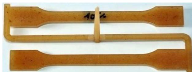
Fig. 3. Injection molded piece made of WPC (10 vol.% WF)
