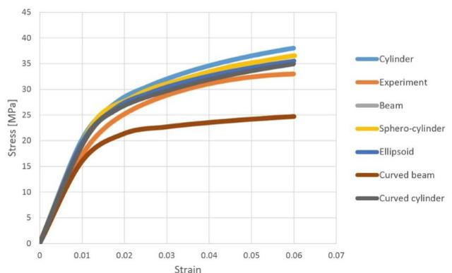
Fig. 8. Calculated stress-strain characteristics of WPC for various shapes of wood fibers compared with experiment result
