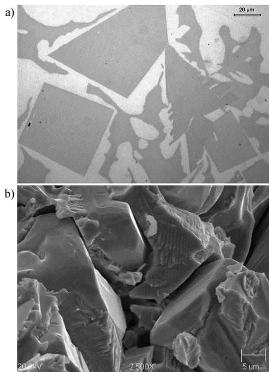
Fig. 3. Microstructure of Ni<sub>3</sub>Al/WC composite, 500x, (a) and scanning image of Ni<sub>3</sub>Al/WC composite fracture, 2500x (b)
