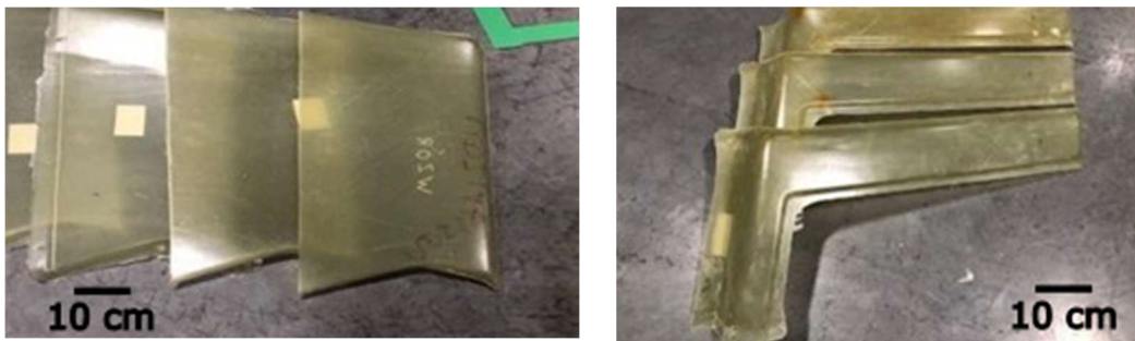
Figure 10. TRIGGO car body parts made in single-sided heated mold in membrane press with vacuum bag assistance, from left: casing, casing_C_right.
