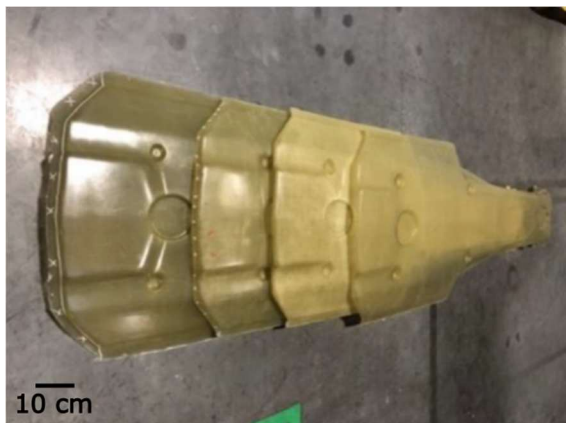
Figure 9. TRIGGO vehicle parts made in single-sided heated mold in membrane press with membrane vacuum assistance (casing bottom).
