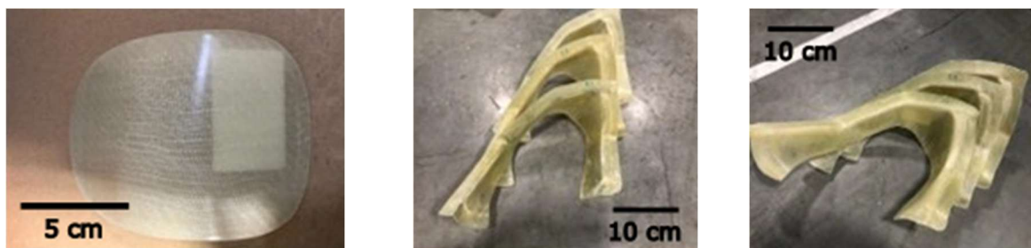
Figure 7. TRIGGO body parts made in single-sided mold heated in vacuum-assisted oven using bag, from left: hatch, cowl_D_Left, cowl_D_Right.
