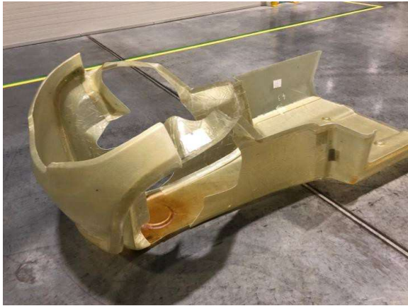
Figure 12. TRIGGO body parts fabricated as part of the project, connected in layout that matches assumptions.
