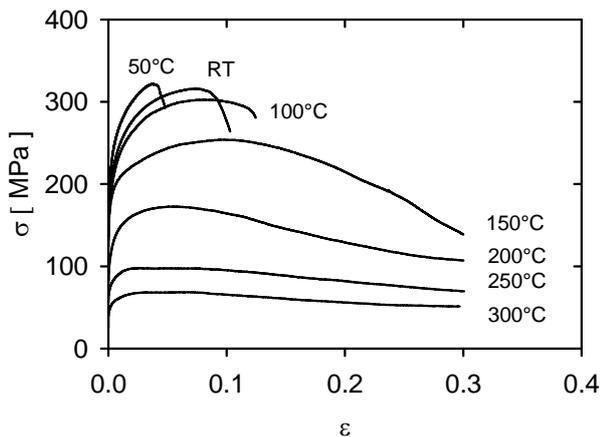
Fig. 10. True stress-true strain curves for QE22/Al<sub>2</sub>O<sub>3</sub>/SiC hybrid in  $\perp$  orientation obtained at various temperatures
