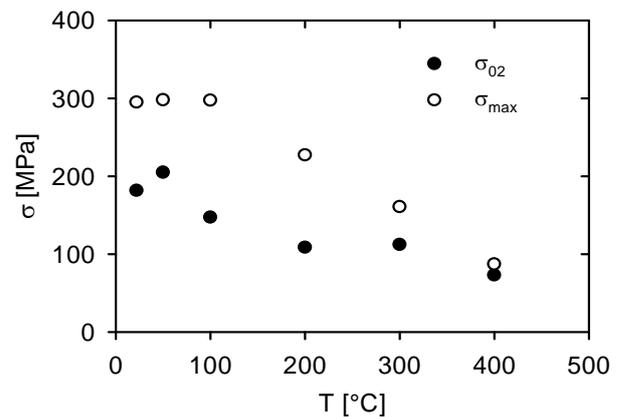
Fig. 7. Temperature dependencies of the characteristic stresses for QE22/Al<sub>2</sub>O<sub>3</sub> in  $\perp$  orientation
