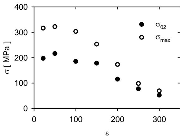
Fig. 11. Temperature dependencies of the characteristic stresses for QE22/Al<sub>2</sub>O<sub>3</sub>/SiC hybrid in  $\perp$  orientation
