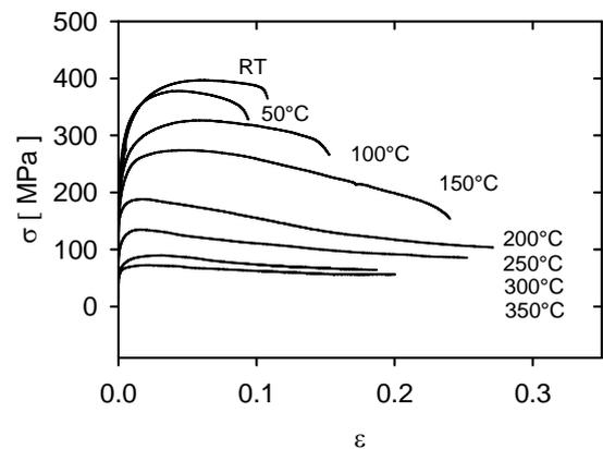
Fig. 8. True stress-true strain curves for QE22 with Saffil fibres and SiC particles in  $\parallel$  orientation obtained at various temperatures
