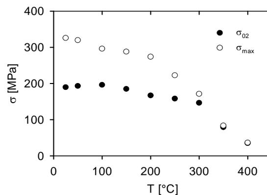
Fig. 3. Temperature dependencies of the characteristic stresses for QE22 unreinforced matrix
