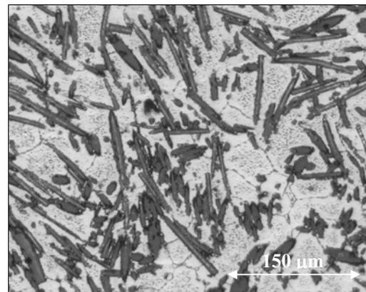
Fig. 13. Saffile fibres in the QE22 matrix. Grain size is smaller in comparison with the matrix alloy
