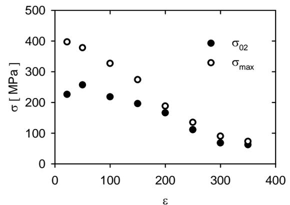
Fig. 9. Temperature dependencies of the characteristic stresses for QE22 with Saffil fibres and SiC particles in  $\parallel$  orientation
