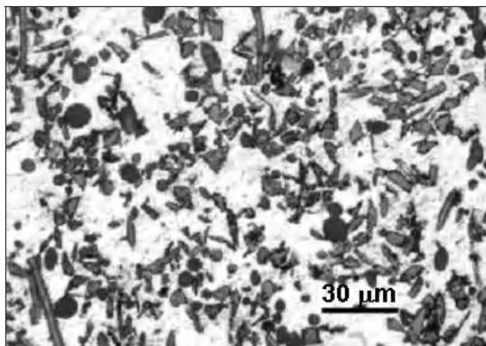
Fig. 1. Microstructure of QE22 hybrid composite (with Saffil fibres and SiC particles)
