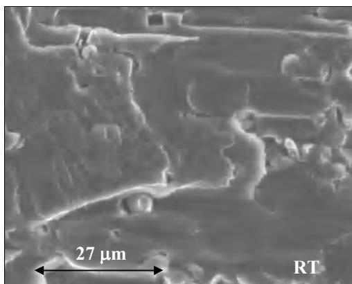
Fig. 14. Fracture surface of hybrid  $\perp$  deformed at RT
