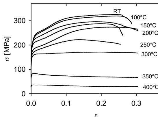
Fig. 2. True stress-true strain curves obtained for the QE22 matrix alloy
