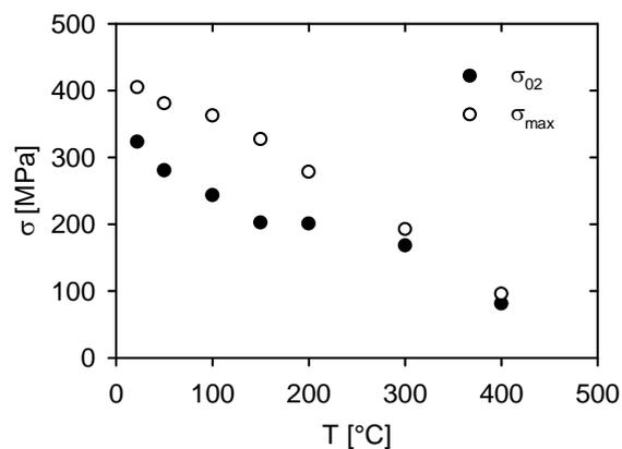
Fig. 5. Temperature dependencies of the characteristic stresses for QE22/Al<sub>2</sub>O<sub>3</sub> in  $\parallel$  orientation
