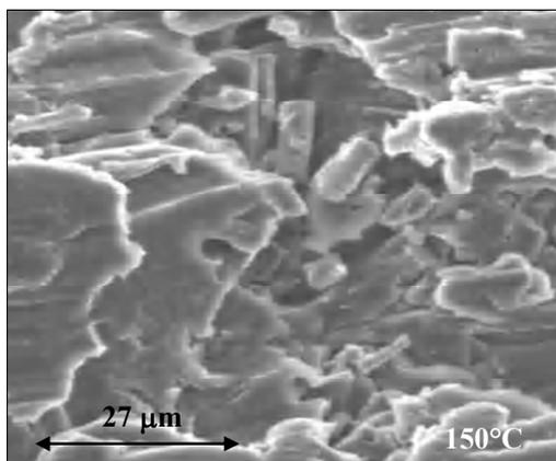
Fig. 15. Fracture surface of hybrid  $\perp$  deformed at 150°C. Debonding of fibers is visible
