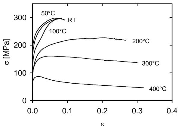
Fig. 6. True stress-true strain curves for QE22/Al<sub>2</sub>O<sub>3</sub> in  $\perp$  orientation obtained at various temperatures
