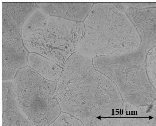
Fig. 12. Microstructure of QE22 monolithic alloy after T6 heat treatment. Grain boundaries and small precipitates are visible
