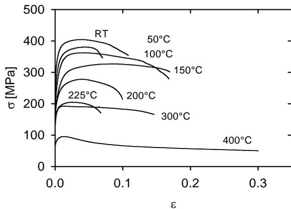
Fig. 4. True stress-true strain curves for QE22/Al<sub>2</sub>O<sub>3</sub> in  $\parallel$  orientation obtained at various temperatures
