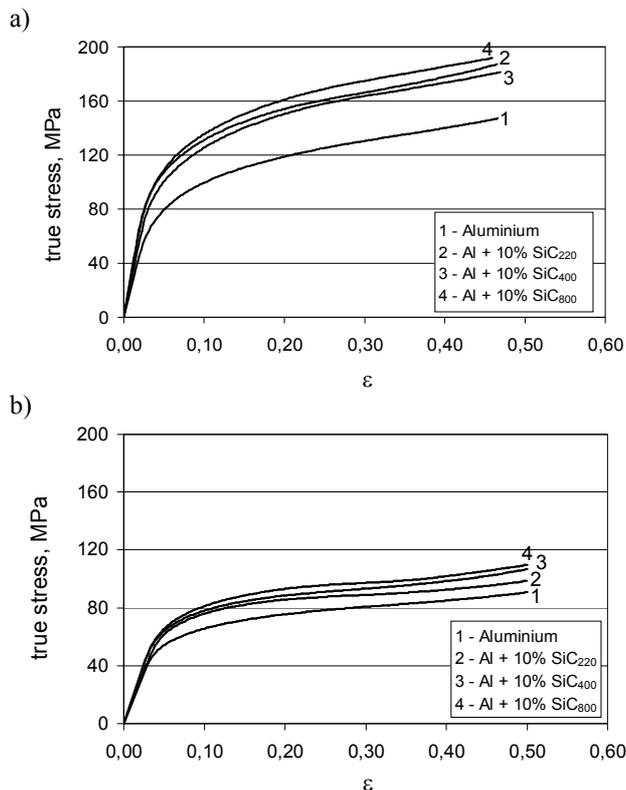
Fig. 2. Influence of chemical composition and size of reinforcing phase particles on character of true stress-strain curves obtained in compression test at room temperature (a) and at 200°C (b), for hot-extruded samples of aluminium and Al-based composites reinforced with 10 % silicon carbide particles
