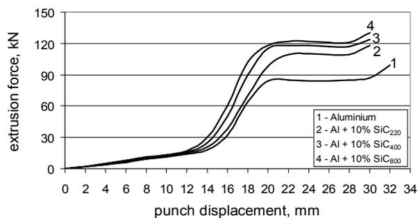
Fig. 1. Extrusion forces during hot extrusion as function of punch displacement
