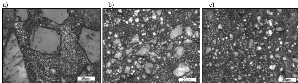
Fig. 4. Microstructures of hot-extruded aluminium-based composites reinforced with 10% particles: a) SiC<sub>220</sub>, b) - SiC<sub>400</sub>, c) SiC<sub>800</sub>. Longitudinal polished sections
