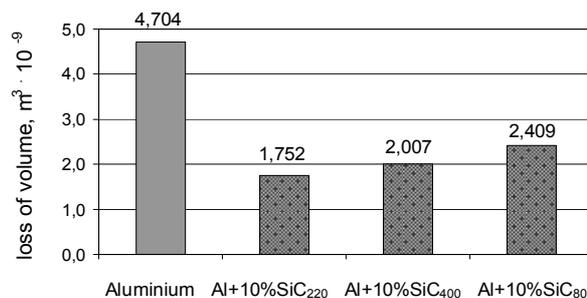
Fig. 3. Influence of chemical composition and particle size on abrasive wear of samples extruded at 500°C, produced from aluminium and composites reinforced with 10% silicon carbide particles
