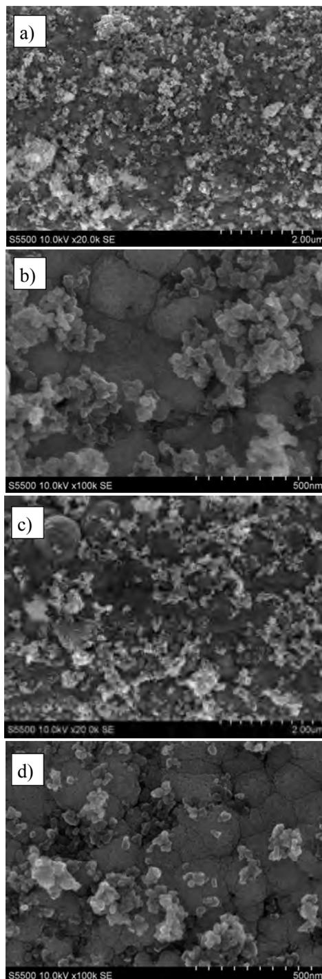
Fig. 1. Composite layer of Ni-P/TiO<sub>2</sub> on carbon fiber substrate obtained from glycine solution with pH 8.5, deposition time 5 min: a,b) TiO<sub>2</sub> concentration 10 g/l; c,d) 30 g/l TiO<sub>2</sub>
