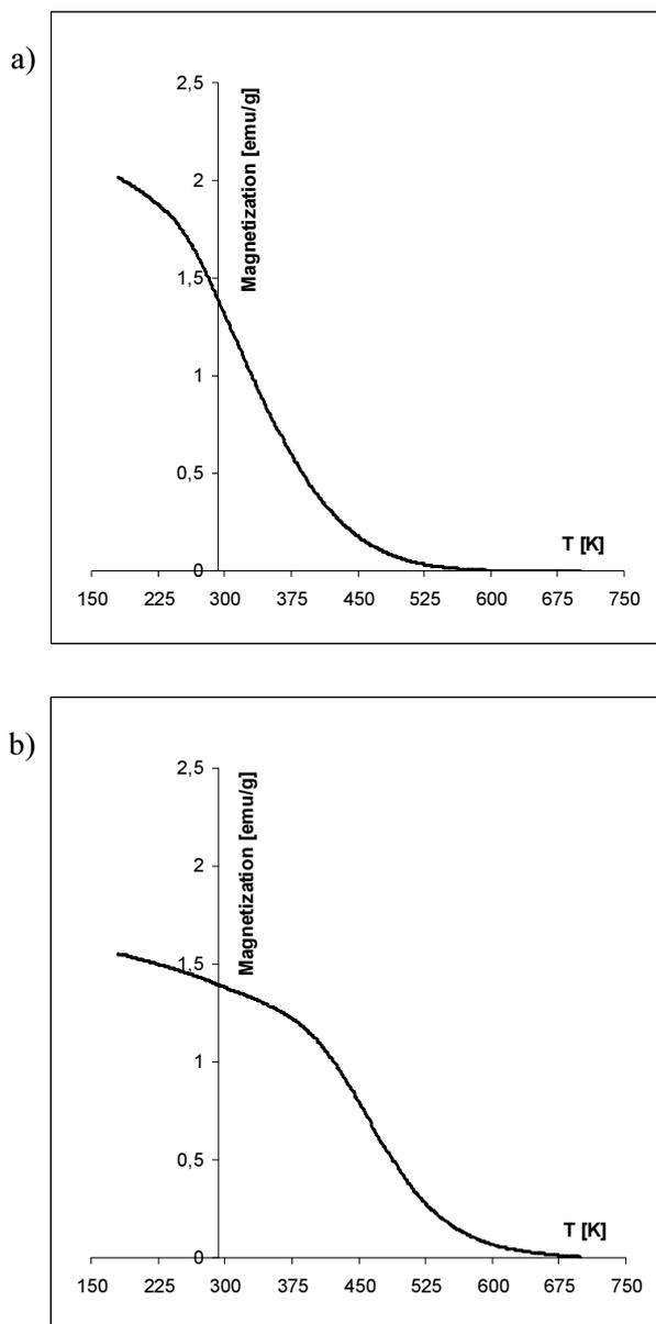
Fig. 3. Plots of (mass)magnetization [emu/g] vs. temperature [K] for: a) W90.3Ni7Fe1.7Co1, b) W90Ni4Fe2Mo4
