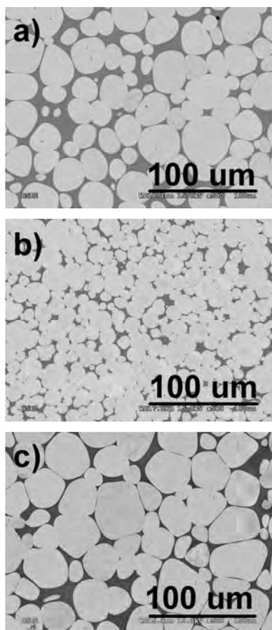
Fig. 1. SEM images of cross sections of: a) W90.3Ni7Fe1.7Co1, b) W90Ni4Fe2Mo4, c) W93Ni5Cu2 composites
