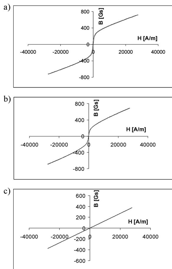
Fig. 2. Magnetic induction  $B$  [Gs] vs. applied field  $H$  [A/m] for: a) W90.3Ni7Fe1.7Co1, b) W90Ni4Fe2Mo4, c) W93Ni5Cu2
