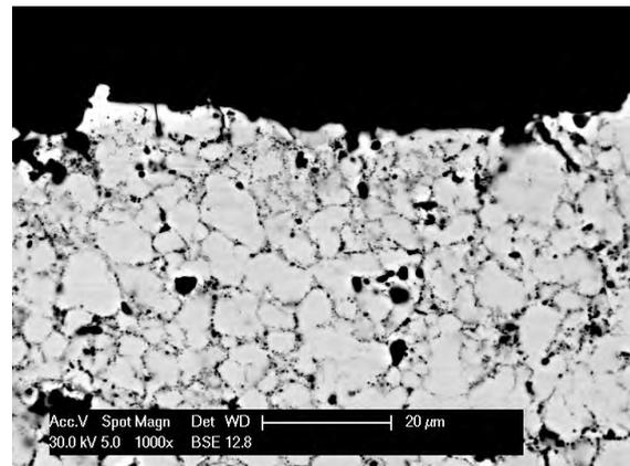
Fig. 3. SEM microstructure of sinter surface after wire electric discharge machining finishing (WEDM) ( $I_A = 40$  A,  $t_p = 100$   $\mu\text{s}$ )
