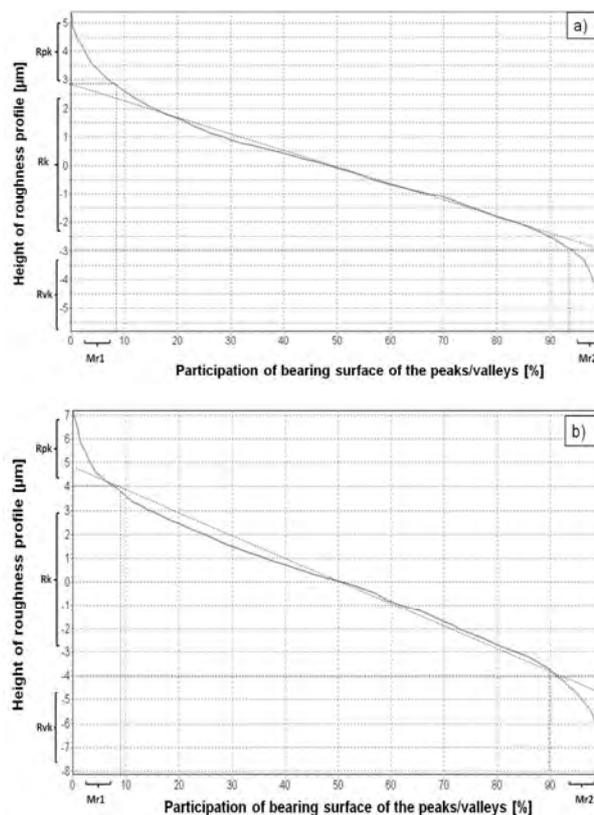
Fig. 6. Load capacity curves of sinters after EDM finishing: a) Fe40Al+2% vol. nAl<sub>2</sub>O<sub>3</sub> ( $I_A = 40$  A,  $t_p = 100 \mu$ s), b) Fe40Al+2% vol. nAl<sub>2</sub>O<sub>3</sub> ( $I_A = 80$  A,  $t_p = 100 \mu$ s)
