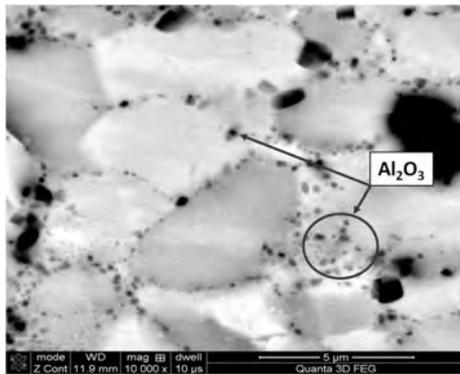
Fig. 1. SEM microstructure of Fe40Al sinter with addition of 2% vol.  $\text{Al}_2\text{O}_3$  [10]
