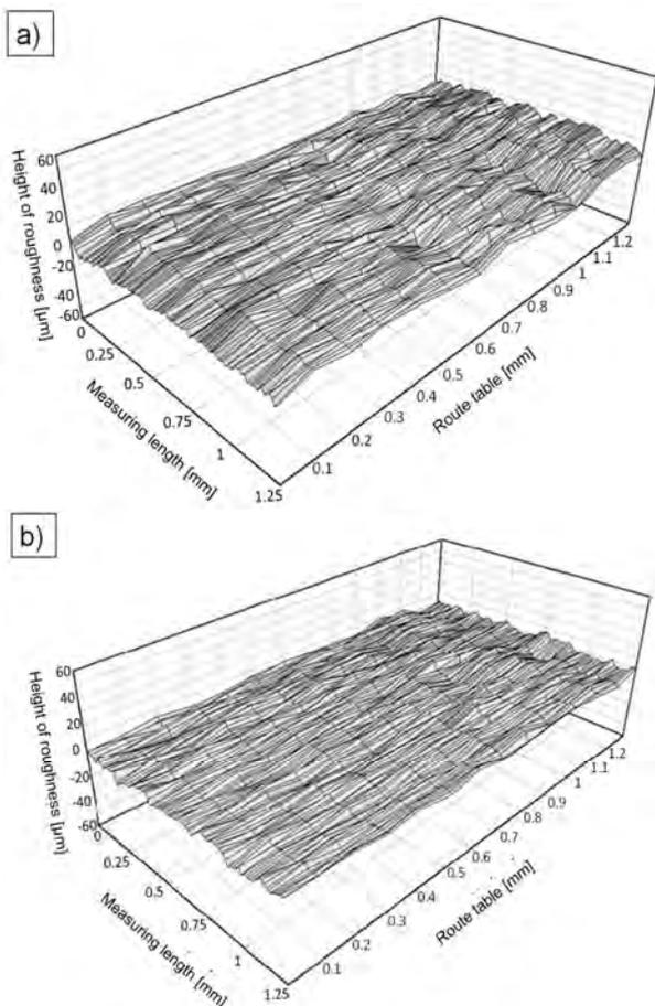
Fig. 5. 3D roughness profile of sinter surface after EDM finishing: a) Fe40Al+2% vol. nAl<sub>2</sub>O<sub>3</sub> ( $I_A = 40$  A,  $t_p = 100 \mu$ s), b) Fe40Al+2% vol. nAl<sub>2</sub>O<sub>3</sub> ( $I_A = 80$  A,  $t_p = 100 \mu$ s)
