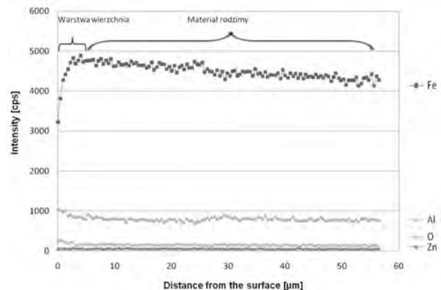
Fig. 4. Linear analysis of chemical composition of surface layer after WEDM ( $I_A = 80$  A,  $t_p = 100$   $\mu\text{s}$ )
