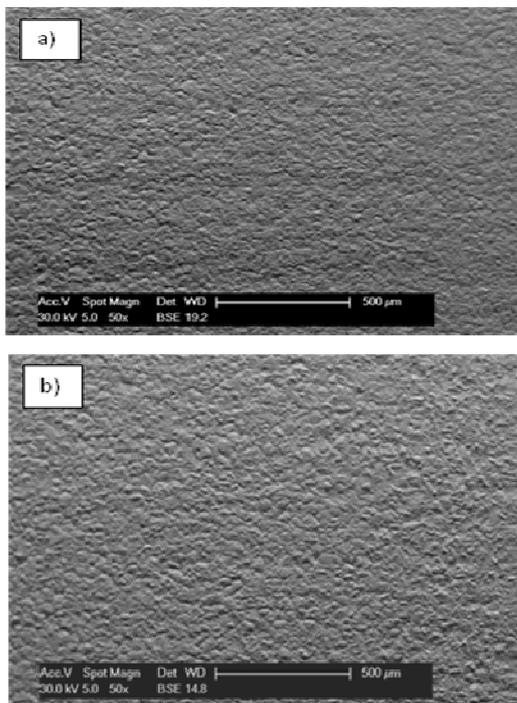
Fig. 2. Surface of sinters after WEDM finishing treatment: a) Fe40Al+2% vol.  $\text{nAl}_2\text{O}_3$  ( $I_A = 40$  A,  $t_p = 100$   $\mu\text{s}$ ), b) Fe40Al+2% vol.  $\text{nAl}_2\text{O}_3$  ( $I_A = 80$  A,  $t_p = 100$   $\mu\text{s}$ )
