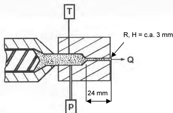
T, P - temperature and mass pressure sensors respectively
